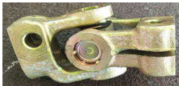
Fig.1 Universal Joint of Tata Sumo
