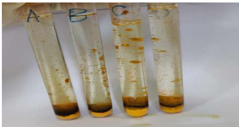
Figure 6: Presence of Lead Salts. Disappearance of Red color on addition of water was observed.
