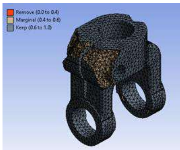
Fig.7 Material to be removed
